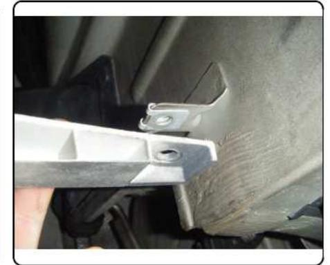
2. Raise nut plate and mounting strap into position around the vehicle crossmember. Secure using 1/2-13 x 2 1/2" hex bolts and 1/2" conical toothed washers.
