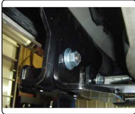
4. Press hitch against the bottom of the bumper beam. (NOTE: Be sure hitch is centered on vehicle.) Using the hitch as a template mark hole locations. Lower hitch and drill marked locations. (NOTE: Start with a small drill bit for pilot hole. A die grinder with a cone shaped bit may be easier than drill bits.)
